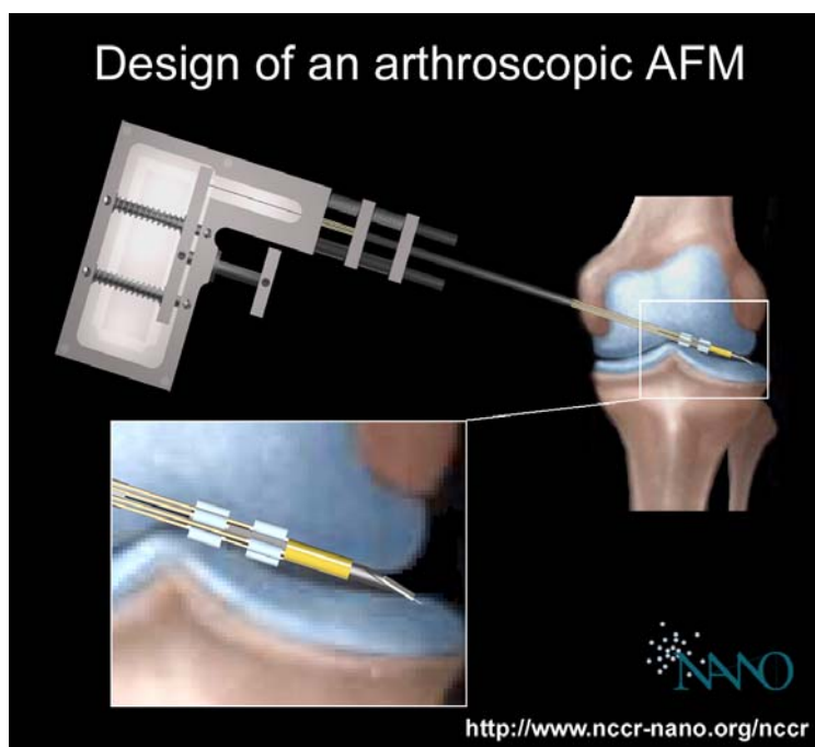
Fig. 1 Illustration of a prototype arthroscopic AFM. The instrument is inserted into the knee cavity under arthroscopic control.
