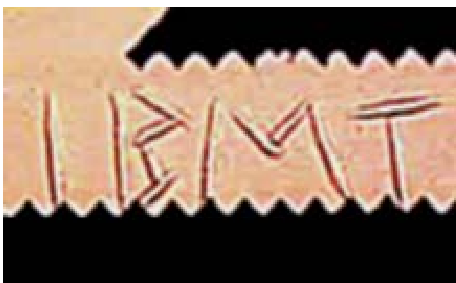
Figure Forisomes (plant protein complexes, length 30 \mu\text{m} ) arranged between electrodes (black) for electrotitration of pH.
